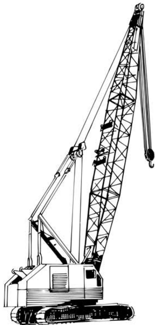
23. Wind on the boom and load can greatly affect the crane's structural strength and stability. **Know the manufacturer's recommended wind speed limitations for the crane you are operating.** You know it's a little too windy when *Stinker starts flying a stunt kite out the cab door.*
