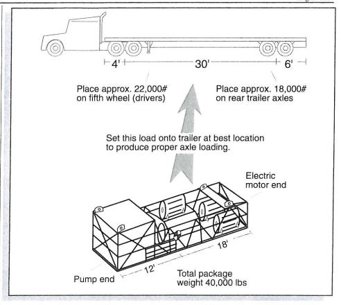
**Assignment:** Place the package where it produces proper loading for the rear and driver axles.
