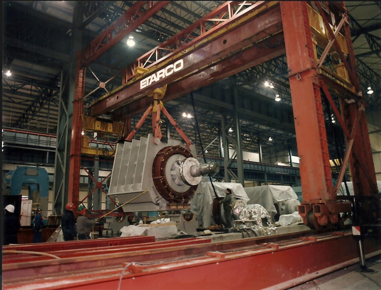
Skid track on top of lift beam for lateral movement
